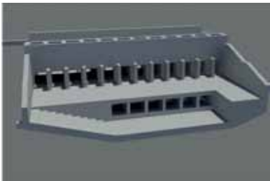
Figure 6.12. The Scheldt side of the inlet and outlet structure. The 3 drainage shafts are visible at the bottom (each shaft consists of 2 sections), and the 6 inlet shafts at the top (also each consisting of 2 sections).
